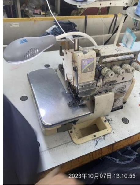
NC closed & respective clause # CA 4: Based on provided evidence, it was noted that the facility installed finger guards and eye guards for all sewing machines.
