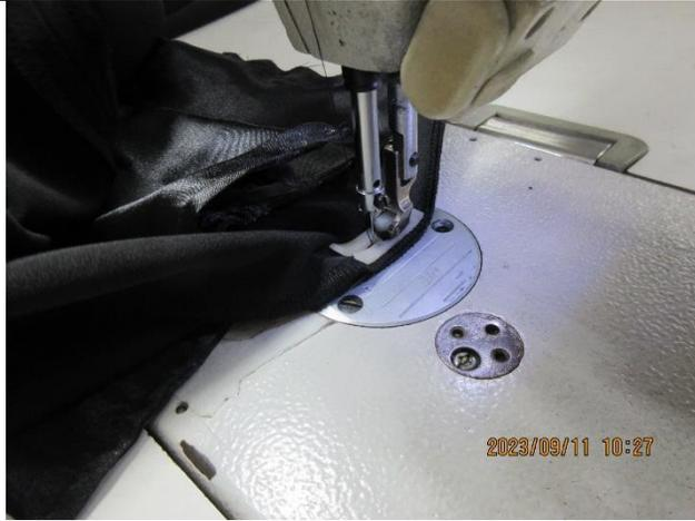
NC raised & respective clause # CA 4: About 10% of sewing equipment in sewing workshop were not installed with finger guards.
